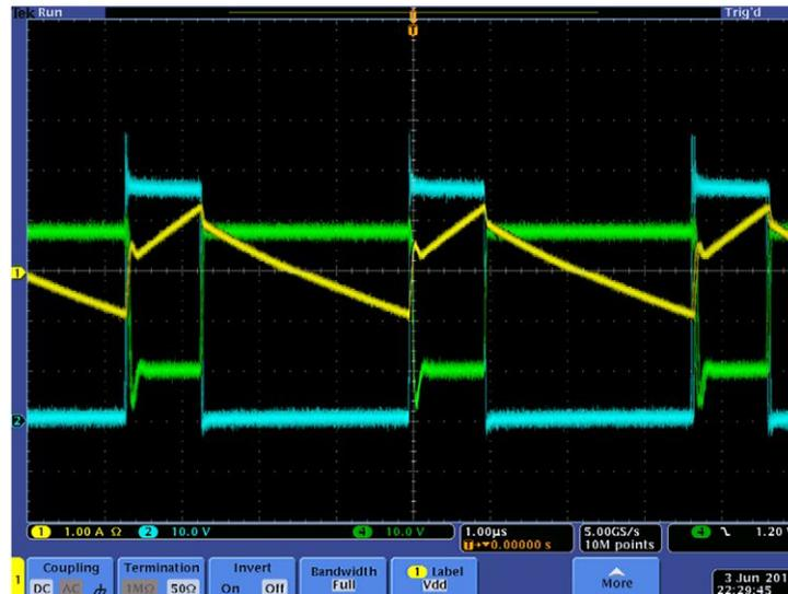
Fig. 7 - Waveform with a full load (1 A) on Iso +5 and 0 A on main +12 at 45 V<sub>IN</sub>
