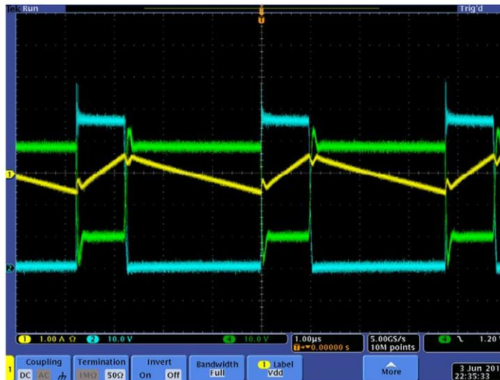
Fig. 5 - Waveform with no load on Iso +5 and 0 A on main +12 45  $V_{IN}$
