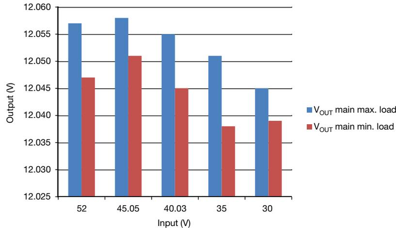
Fig. 10 - Main +12 V output voltage regulation over loading on all outputs and line voltage
