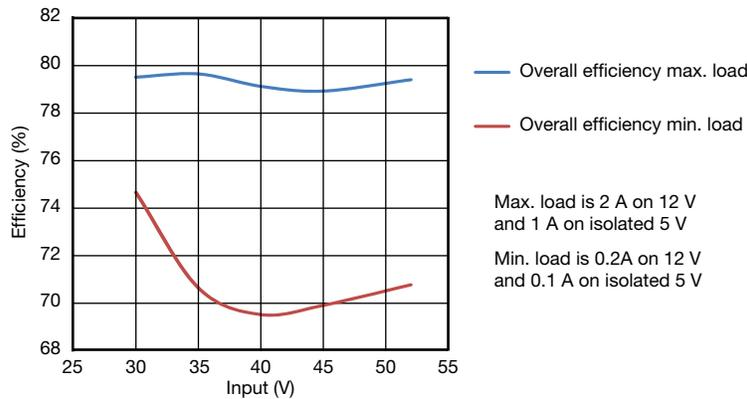
Fig. 9 - Efficiency over the input voltage range and load range (includes secondary switching regulator, U10)
