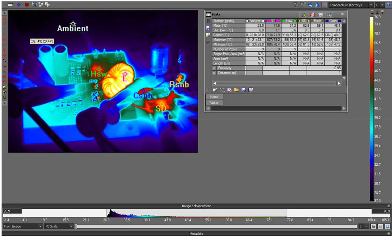
Fig. 12 - Thermal image at 55 V<sub>INPUT</sub> and a full load on both outputs
