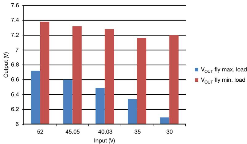
Fig. 11 - Flyback output voltage regulation on C18 over loading on all outputs and line voltage
