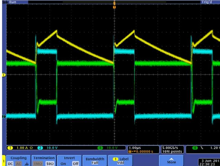
Fig. 8 - Waveform with a full load (1 A) on Iso +5 and 2 A on main +12 45 V<sub>IN</sub>
