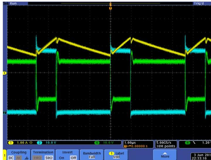
Fig. 6 - Waveform with no load on Iso +5 and 2 A on main +12 at 45 V<sub>IN</sub>
