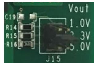
Fig. 2 - J15 Jumper on EVB for Output Voltage Setting
