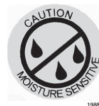
Fig. 9 - Moisture-Sensitive Identification Label (MSID)
