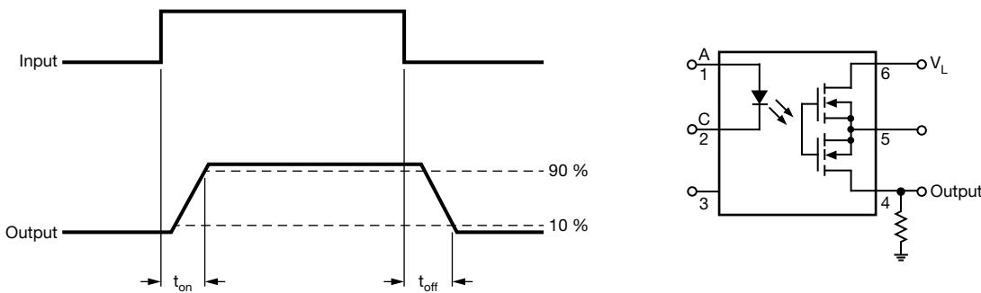
Fig. 2 - Timing Schematic
