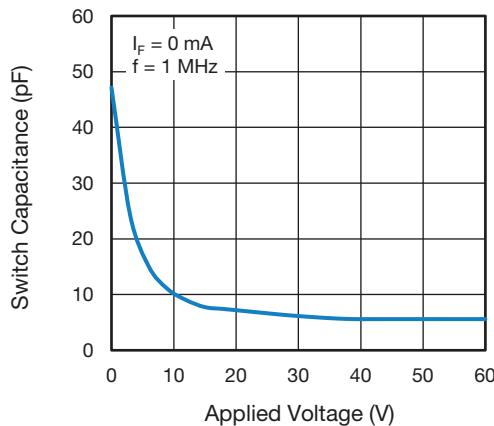
Fig. 10 - Switch Capacitance vs. Applied Voltage
