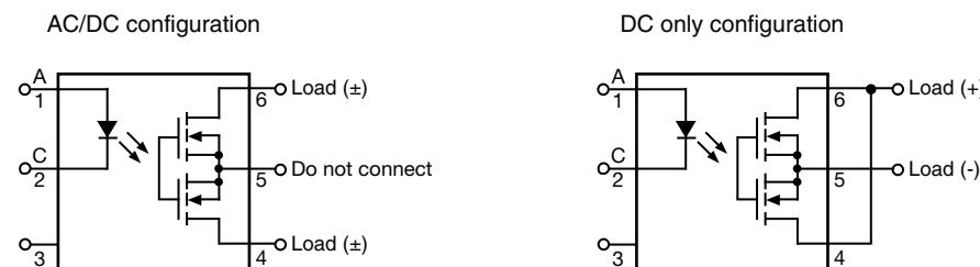
Fig. 1 - Pin Configuration
