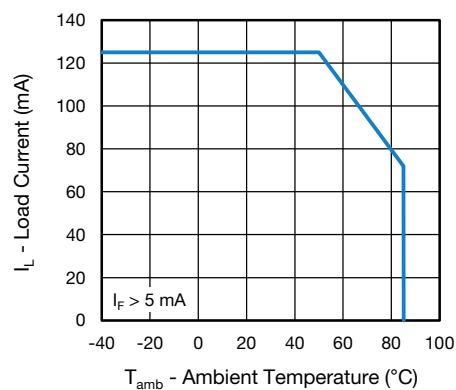
Fig. 5 - Maximum Load Current vs. Ambient Temperature
