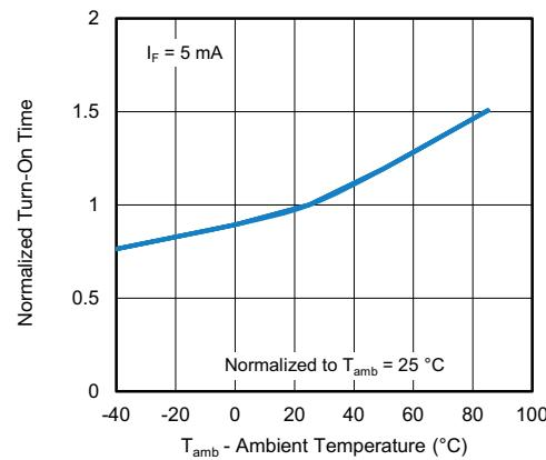
Fig. 13 - Normalized Turn-On Time vs. Ambient Temperature
