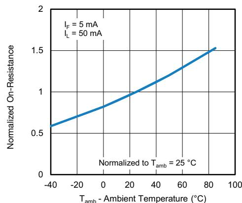
Fig. 9 - Normalized On-Resistance vs. Ambient Temperature
