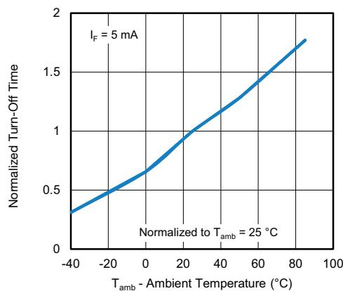
Fig. 15 - Normalized Turn-Off Time vs. Ambient Temperature
