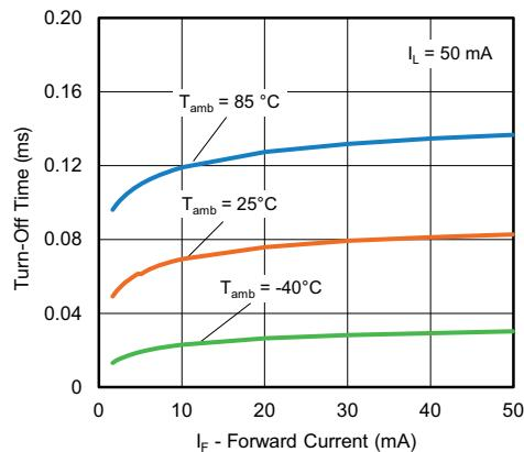
Fig. 13 - Turn-Off Time vs. Forward Current
