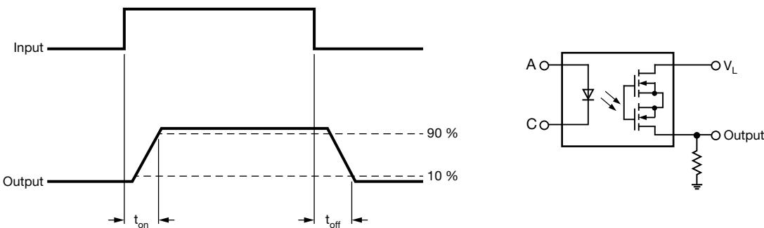
Fig. 1 - Timing Schematic
