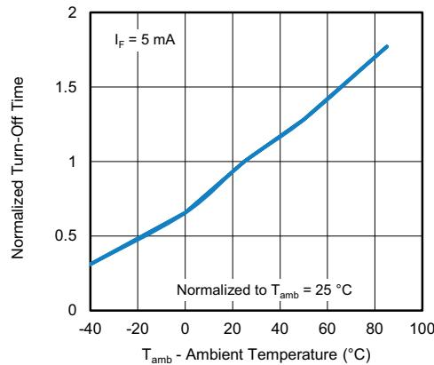
Fig. 14 - Normalized Turn-Off Time vs. Ambient Temperature
