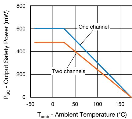
Fig. 2 - Safety Power Dissipation vs. Ambient Temperature
