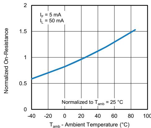
Fig. 8 - Normalized On-Resistance vs. Ambient Temperature
