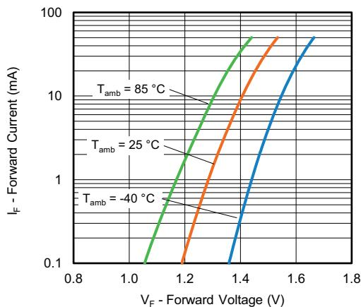
Fig. 6 - Forward Current vs. Forward Voltage
