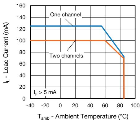
Fig. 4 - Maximum Load Current vs. Ambient Temperature
