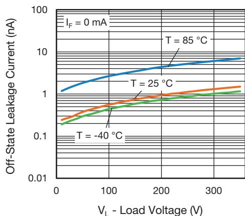
Fig. 10 - Off-State Leakage Current vs. Load Voltage
