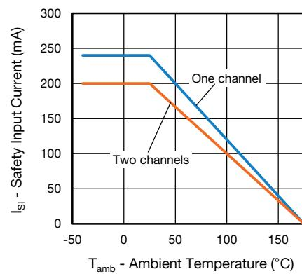
Fig. 3 - Safety Input Current vs. Ambient Temperature
