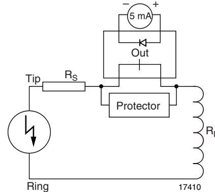
Fig. 2 - Test Setup with Protector across SSR Contacts
