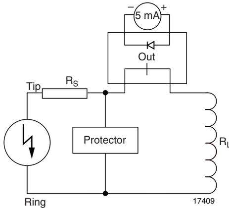
Fig. 1 - Test Setup with Protector across Tip to Ring
