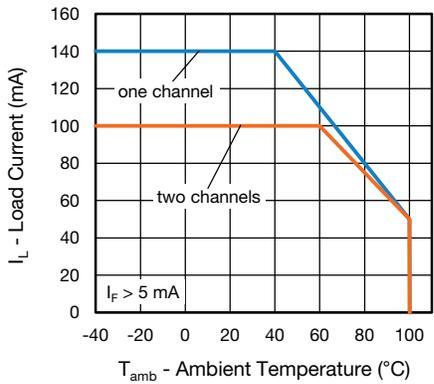
Fig. 4 - Maximum Load Current vs. Ambient Temperature
