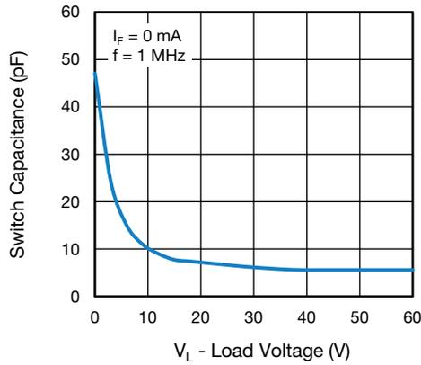
Fig. 9 - Output Capacitance vs. Load Voltage
