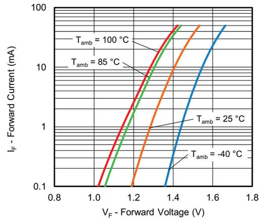
Fig. 6 - Forward Current vs. Forward Voltage
