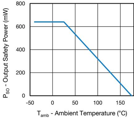
Fig. 2 - Safety Power Dissipation vs. Ambient Temperature
