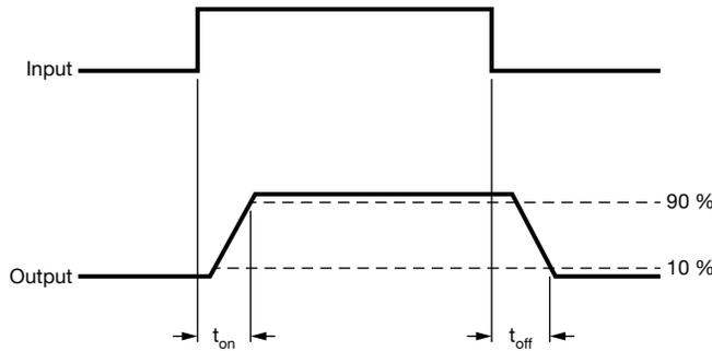
Fig. 1 - Timing Schematic
