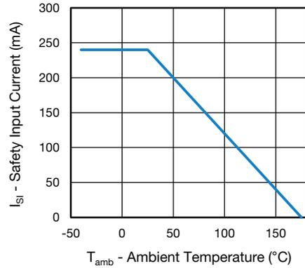
Fig. 3 - Safety Input Current vs. Ambient Temperature
