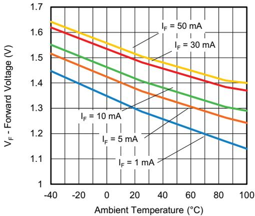
Fig. 5 - Forward Voltage vs. Ambient Temperature
