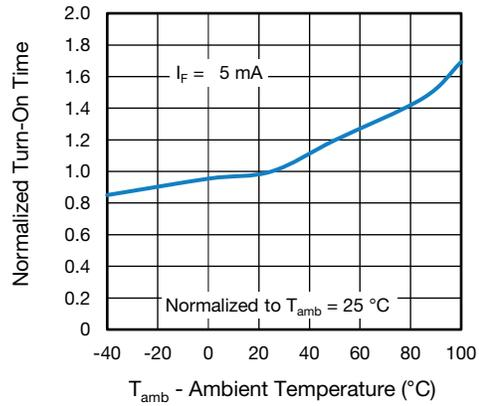
Fig. 12 - Normalized Turn-On Time vs. Ambient Temperature
