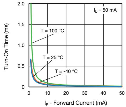
Fig. 11 - Turn-On Time vs. Forward Current
