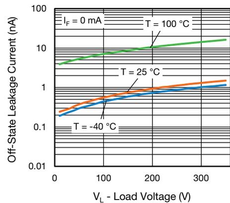
Fig. 10 - Off-State Leakage Current vs. Load Voltage
