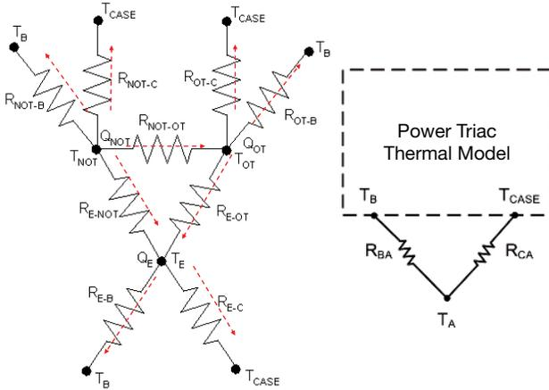
Fig. 3 - Three Dice Power Phototriac Thermal Model/Resistor Network
