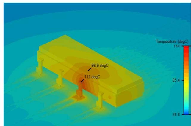
Fig. 2 - Example of Package Temperature Profile (4-Layer Board)
