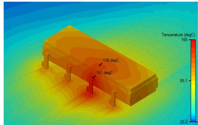
Fig. 1 - Example of Package Temperature Profile (2-Layer Board)
