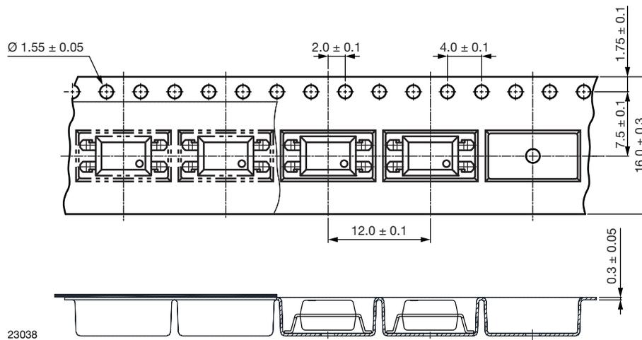
Fig. 16 - Tape and Reel Packaging (1000 pieces on reel)
