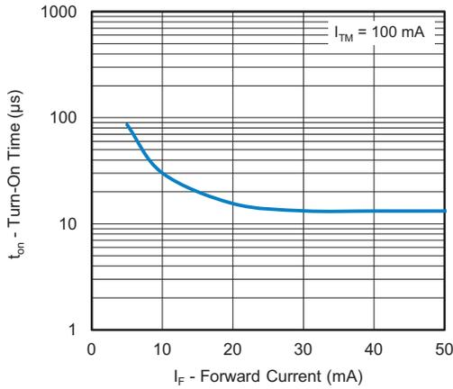
Fig. 9 - Turn-On Time vs. Forward Current
