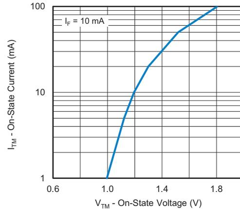
Fig. 6 - On State Current vs. On State Voltage
