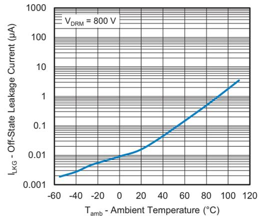
Fig. 8 - Off-State Leakage Current vs. Ambient Temperature
