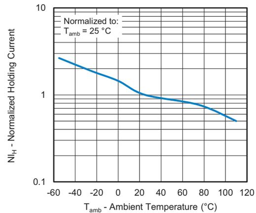
Fig. 7 - Normalized Holding Current vs. Ambient Temperature
