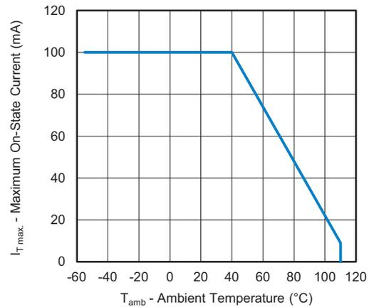
Fig. 2 - Maximum On-State Current vs. Ambient Temperature
