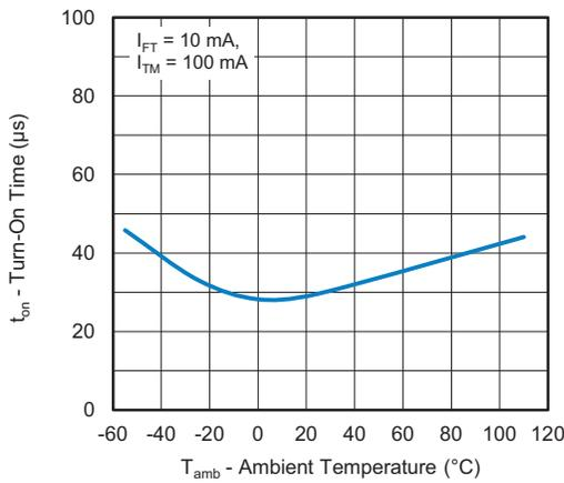
Fig. 10 - Turn-On Time vs. Ambient Temperature
