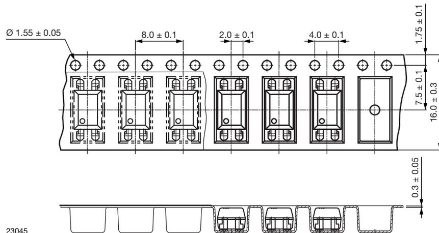
Fig. 17 - Tape and Reel Packaging (2000 pieces on reel)
