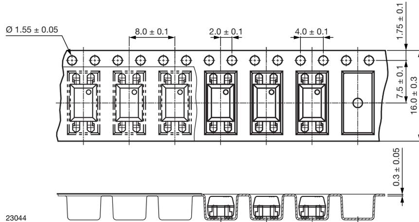
Fig. 15 - Tape and Reel Packaging (2000 pieces on reel)
