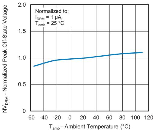
Fig. 11 - Normalized Peak Off-State Voltage vs. Ambient Temperature
