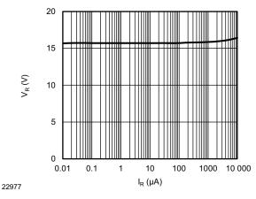
Fig. 3 - Typical Reverse Voltage vs. Reverse Current
