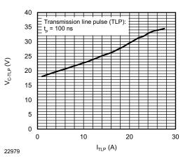
Fig. 5 - Typical Clamping Voltage vs. Peak Pulse Current
