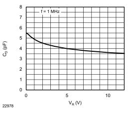
Fig. 4 - Typical Capacitance vs. Reverse Voltage
