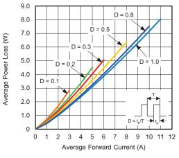
Fig. 2 - Forward Power Loss Characteristics
