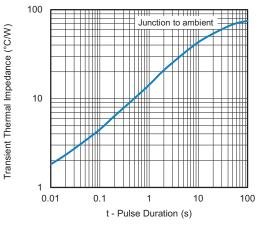
Fig. 6 - Typical Transient Thermal Impedance
