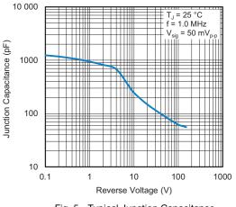
Fig. 5 - Typical Junction Capacitance
