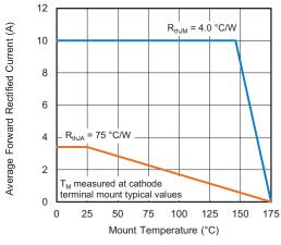
Fig. 1 - Forward Current Derating Curve
