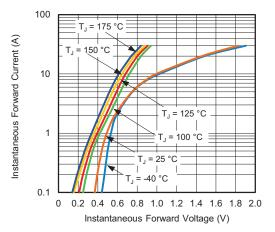
Fig. 3 - Typical Instantaneous Forward Characteristics
