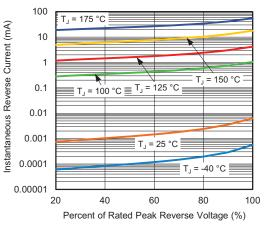
Fig. 4 - Typical Reverse Leakage Characteristics Per Diode
