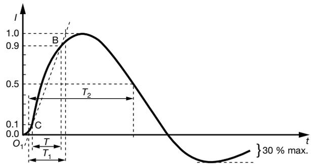
Front time:  $T_1 = 1.25 \times T = 8 \mu\text{s} \pm 20\%$
