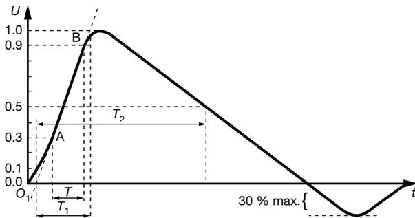
Front time:  $T_1 = 1.67 \times T = 1.2 \mu\text{s} \pm 30\%$
