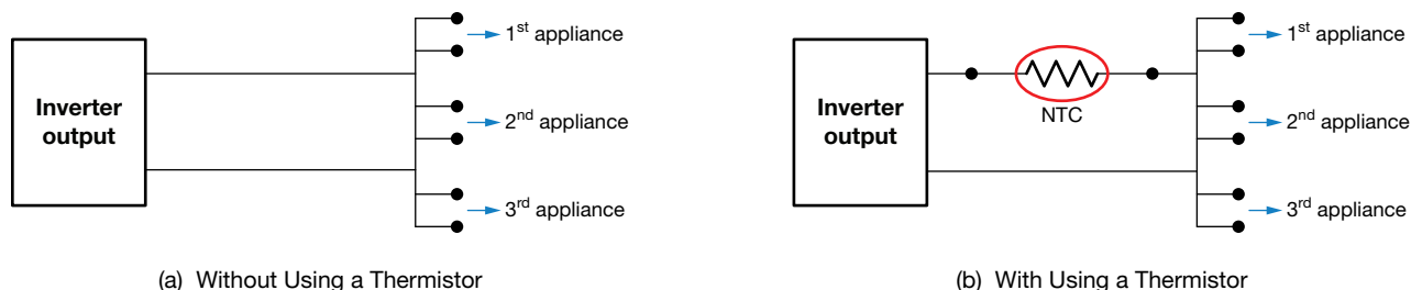
Fig. 4 - Inverter Inrush Overload Diagram
