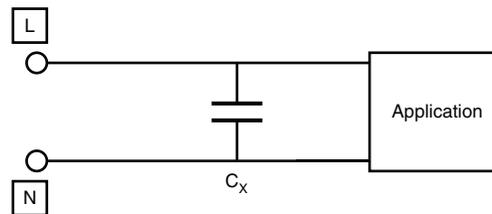
Several functions are combined in these small components: excellent high frequency properties for short circuiting radio interference, the ability to withstand continuous stress from the AC mains voltage, and the ability to sustain transient voltages - caused, for example, by lightning strikes and switching - superimposed on the line.
