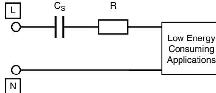
In this application, capacitors are connected in series to the mains and the functions to be fulfilled are:
