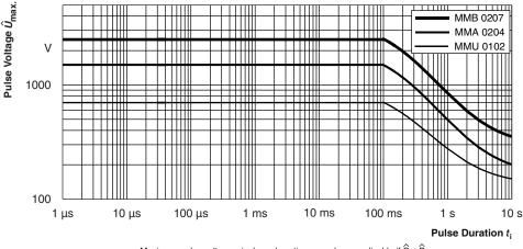
$\begin{array}{l} \mbox{Maximum pulse voltage, single and continuous pulses; applicable if $\widehat{P} \leq \widehat{P}_{max}$; $$ for permissible resistance change $\pm$ (0.5 % $R$ + 0.01 $\Omega$) $ \end{array}$
