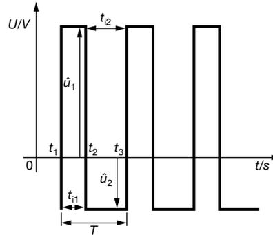
$$P_{\text{rec}} = \frac{1}{T} \times \frac{1}{R} \times (\hat{u}_1^2 \times t_{i1} + \hat{u}_2^2 \times t_{i2})$$
