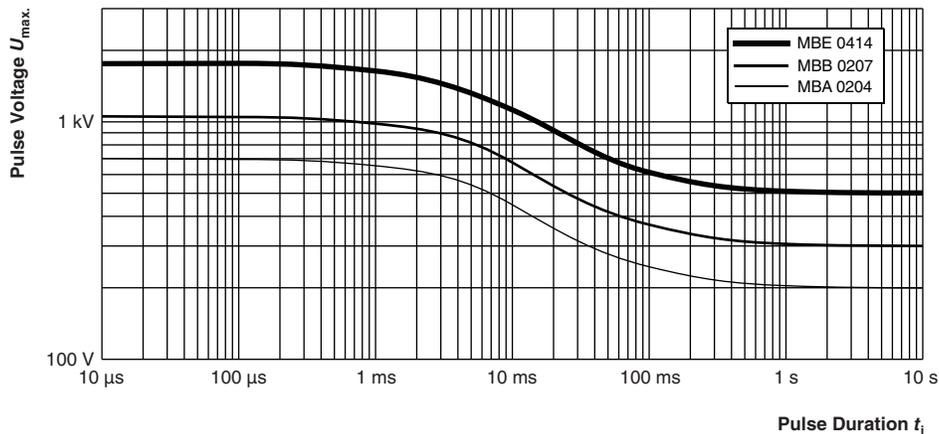
Fig. 4 - Maximum pulse voltage, single and continuous pulses
