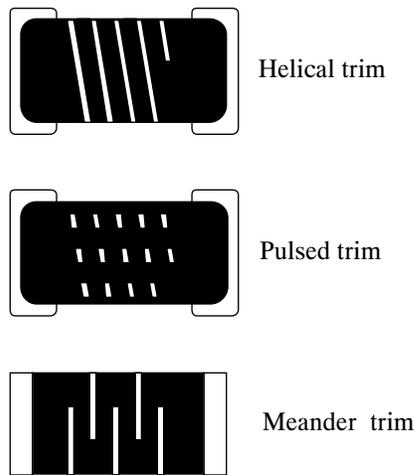
Fig. 3 - Trimming of MELF, MELF HF and Chip
