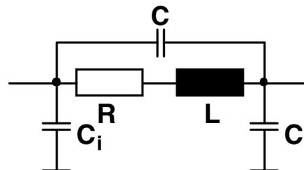
Fig. 2 - Resistor substitution circuit
