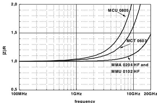
Fig. 5 -  $|Z|/R$  for 50 Ω resistors
