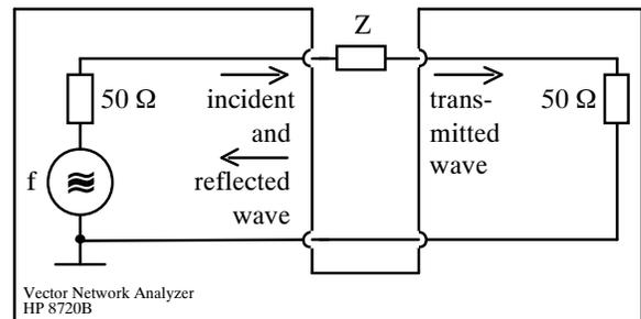
Fig. 4 Reflection and transmission measurement
