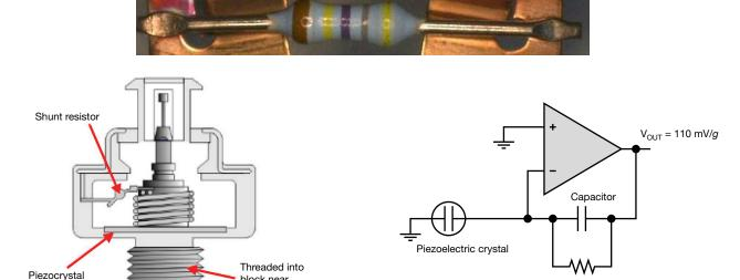
The output voltage is typically 110 mV/g, where "g" is vibration represented in terms of acceleration due to gravity ( $g = 9.8 \text{ m/s}^2$ ). As the vibration intensity increases, such as 2 g or 3 g, the mV signal increases correspondingly.
