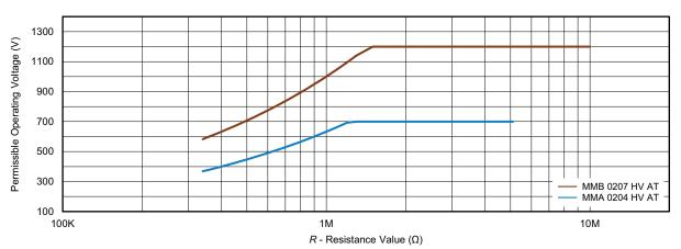
The permissible operating voltage equals the rated voltage  $U_{\rm R}=\sqrt{P_{70}\,{\rm x}\,R}.$  For ambient temperatures above 70 °C power derating must be considered
