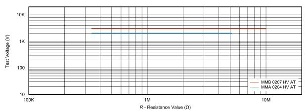
Pulse load rating in accordance with IEC 60115-1, 8.2; 10  $\mu$ s/700  $\mu$ s; 10 pulses at 1 minute intervals; for permissible resistance change  $\pm$  (0.5 % R + 0.05  $\Omega$ )
