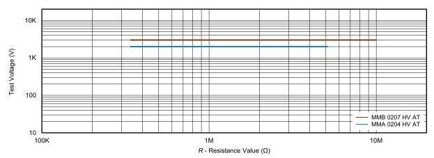
Pulse load rating in accordance with IEC 60115-1, 8.2; 1.2 µs/50 µs; 5 pulses at 12 s intervals; for permissible resistance change  $\pm$  (0.5 % R + 0.05  $\Omega)$
