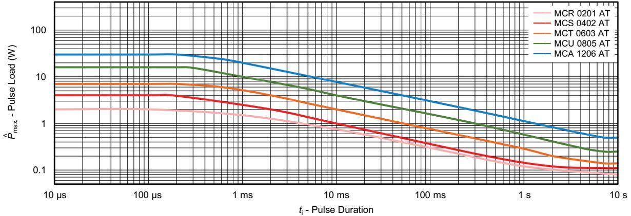
Maximum pulse load, single pulse; applicable if  $\bar{P} \rightarrow 0$  and  $n \leq 1000$  and  $\dot{U} \leq \dot{U}_{max}$ ; for permissible resistance change  $\pm (0.5 \% R + 0.05 \Omega)$
