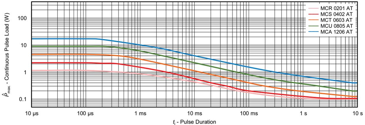
Maximum pulse load, continuous pulse; applicable if  $\bar{P} \leq P(\vartheta_{amb})$  and  $\dot{U} \leq \dot{U}_{max}$ ; for permissible resistance change  $\pm (0.5 \% R + 0.05 \Omega)$
