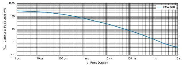
Maximum pulse load, continuous pulse; applicable if  $\overline{P} \le P$  ( $v_{amb}$ ) and  $\hat{U} \le 2$  kV; for permissible resistance change  $\pm$  (0.5 % R + 0.05  $\Omega$ )
