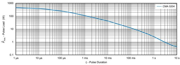
Maximum pulse load, single pulse; applicable if  $\overline{P} \to 0$  and n  $\leq$  1000 and  $\hat{U} \leq$  2 kV; for permissible resistance change  $\pm$  (0.5 % R + 0.05  $\Omega$ )
