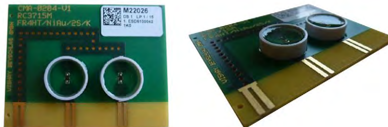
Customized ESD test PCBs: resistors fully encapsulated with epoxy resin
