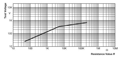
Pulse load rating for arrays with equal values, design type AE, in accordance with EN 60115-1 clause 4.27; 1.2  $\mu$ s/50  $\mu$ s; 5 pulses at 12 s interval; for permissible resistance change (0.5 % R + 0.05  $\Omega$ )
