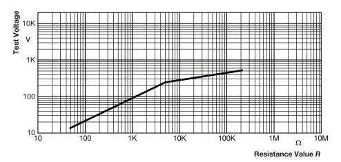
Pulse load rating for arrays with equal values, design type AE in accordance with EN 60115-1 clause 4.27;  $10 \mu s/700 \mu s$ ; 10 pulses at 1 min intervals; for permissible resistance change (0.5 % R + 0.05  $\Omega$ )
