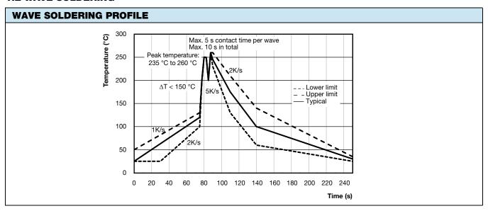
The maximum wave temperature should be limited to 260 °C at all times and the total wave immersion time should be limited to 10 s max. In the case of double wave soldering, the total soldering time, including the time between waves, should also be limited to 10 s max.
