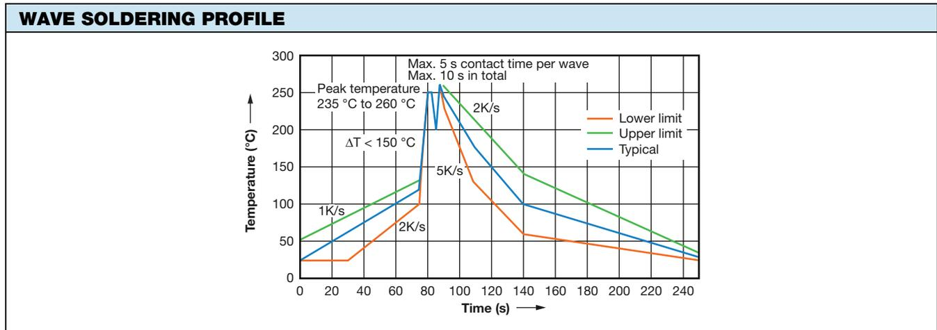
The maximum wave temperature should always be limited to 260 °C, and the total wave immersion time should be limited to 10 s max. In the case of double wave soldering, the total soldering time, including the time between waves, should also be limited to 10 s max.
