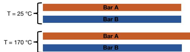
This also applies to a resistor in that the lower TCR will result in a more stable measurement across temperature, which may be caused by applied power (causing the resistance element temperature to increase) or ambient environment.
