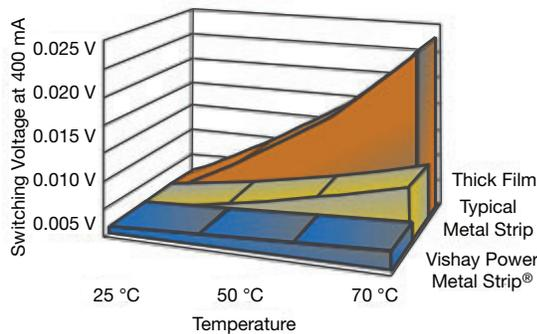
The Power Metal Strip resistor series uses a solid copper terminal (item 2 in the illustration) that is electron beam welded to a low TCR resistance alloy (item 1), achieving low values down to 0.1 mΩ with low TCR. However, the copper terminal has a high TCR (3900 ppm/°C) compared to the resistance alloy (< 20 ppm/°C), which still plays a role in the overall TCR performance as lower resistance values are required.
