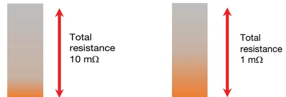
This influence may occur at different resistance value ranges for different parts. For example, the TCR rating of the [WSLP2512](#) is 275 ppm/°C at 1 mΩ, while the [WSLF2512](#) is 170 ppm/°C at 1 mΩ. The WSLF has a lower TCR because the copper terminal has a lower resistance contribution for the same resistance value.
