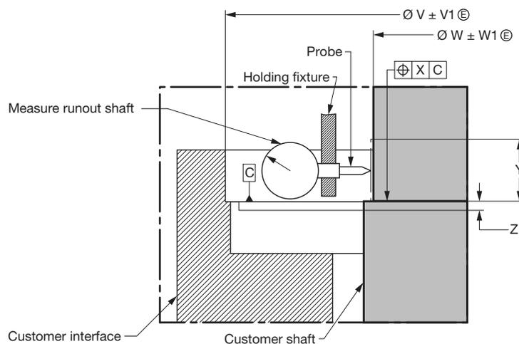
Fig. 2 - Rotor's shaft radial runout
