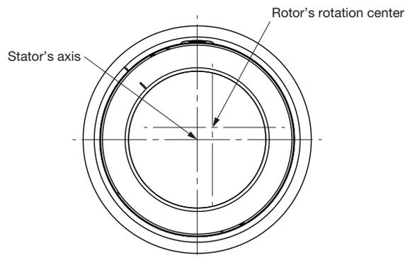
Fig. 12 - Stator's misalignment vs rotor's rotation center
