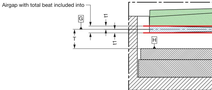
Fig. 7 - Airgap between magnet's top and magnetic cells top
