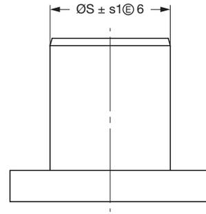
Fig. 4 - Rotor's shaft diameter
