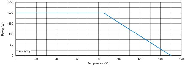
Permanent applicable power (W) as a function of bottom case temperature (°C)
