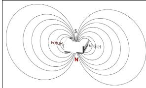
When a positive (+) voltage is placed on the terminal marked with the polarity dot and the opposite terminal is negative (-), the resulting current flow will create a magnetic south pole on the top side of the IHLP. For the IHLE-4040DDEW-5A series, the polarity mark also indicates the "start" or "inside"lead of the winding. Observing the polarity orientation when mounting the IHLP will insure the most consistent EMI reduction performance.
