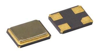
The XT22 series is an ultra miniature package crystal with dimensions 2.5 mm  $\times$  2.0 mm  $\times$  0.65 mm. It is primarily used in notebook, mobile communications, telecom devices, industrial controls, and consumer platforms.
