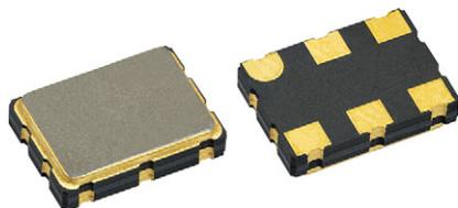
The XO-57L series is an ultra miniature package clock oscillator with dimensions 7.0 mm x 5.0 mm x 1.8 mm. It is specifically developed for telecommunications and network applications like OC-48 and OC-192.
