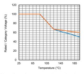
Most of tantalum wet capacitors series do not require voltage derating when used below +85 °C. But DC working voltage (bias) should be chosen so that the sum of the DC bias and AC (ripple) voltages not to exceed the RV. For increased reliability it is recommended to have 10 % to 20 % guard band, meaning not to exceed 80 % to 90 % of RV below +85 °C; at higher temperatures same ratio should be kept with respect to the category voltage.
