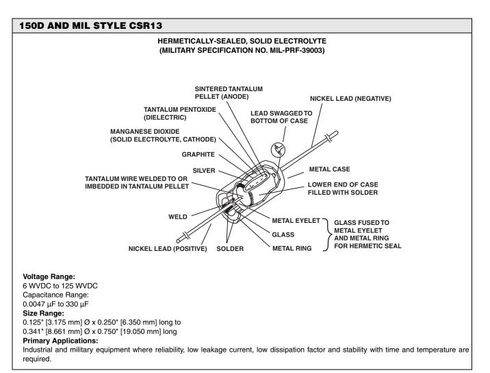
In the tantalum electrolytic capacitor, the distance between the plates is very small since it is only the thickness of the tantalum pentoxide film. As the dielectric constant of the tantalum pentoxide is high, the capacitance of a tantalum capacitor is high if the area of the plates is large:
