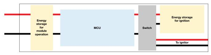
Depending on the design, one or two energy storage capacitors provide ignition. Thus, the capacitor plays an important role. However, with a variety of capacitive technologies available, which is the best for electronic detonators?
