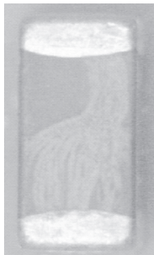
Figure 4. Carbon traces from surface arc-over on a typical Standard High Voltage MLCC
