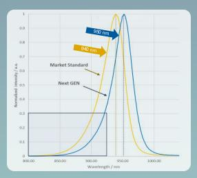
The upgraded wavelength of 950 nm instead of 940 nm reduces the visibility of the IR emitter by the human eye drastically. No red glow and distraction to driver is crucial in driver monitoring!
