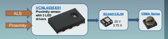
Our VCNL4035 has three integrated LED driver that can be used to at the same time control the driver monitoring emitters and also check the reflection intensity towards the mirror. If a passenger comes too close with their face the proximity sensor can automatically reduce the emitter intensity to avoid any danger to the eye.
