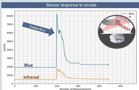
The ratio between the blue light and IR light response can be used to determine whether it is smoke or steam, such as from cooking. Typically, smoke has a higher ratio of IR reflection due to the larger particle sizes present in fire smoke.
