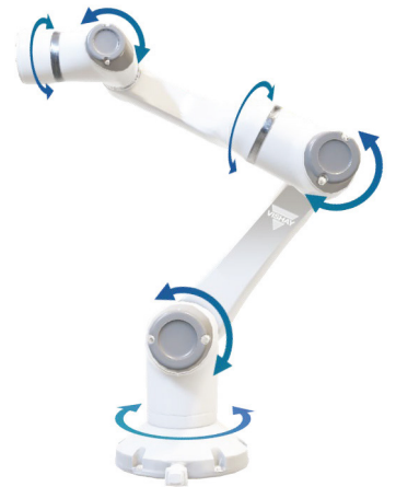
Fig. 01 - Industrial Robot With Multiple Rotational Axes
