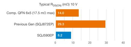
The typical  $R_{DS(ON)}$  of the SQJ590EP is 12.8 % lower than the next best product in the 6 mm by 5 mm package. Compared to a device using the previous-generation technology (SQJ872EP), the  $R_{DS(ON)}$  improvement is 72 %. Maximum junction temperature for all three devices shown above is 175 °C.
