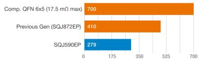
The typical  $R_{DS}^*Q_g$  FOM of the SQJ590EP is 32 % better than the next best product in the 6 mm by 5 mm package. The FOM is improved by 57 % compared to the SQJ872EP.
