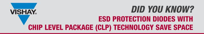
Vishay now offers ESD protection diodes in the ultra compact CLP0603 and CLP1007 packages. The single-line and 4-line ESD protection diodes offer a working range of  $\pm$  3.3 V to  $\pm$  10 V and low leakage current of < 0.1 µA. The devices are ideal for ESD protection of high speed interfaces in smartphones, digital cameras, and gaming systems.
