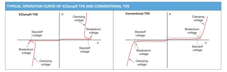
XClampR TVS are snapback type TVS with an extremely low clamping voltage ratio for suppressing transient voltages to lower clamping voltages than conventional TVS.
