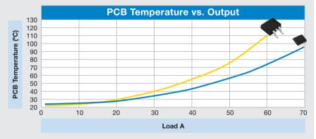
Improved package reduces the device's R<sub>DS(ON)</sub> and leads to lower temperatures at the drain pad of the MOSFET and on the PCB
