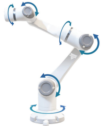
Fig. 01 - Industrial Robot With Multiple Rotational Axes
