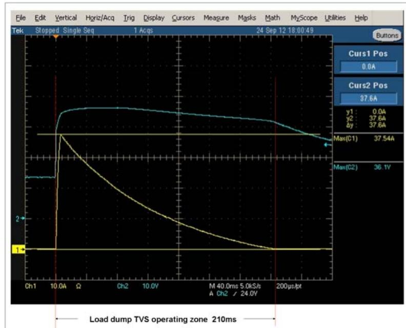
**Figure 2** Clamped waveform of the **SM5S24A** at an ISO-16750-2 pulse: 5A, 101V  $U_s$ ,  $R_i = 1.75\Omega$ , 400ms pulse input condition
