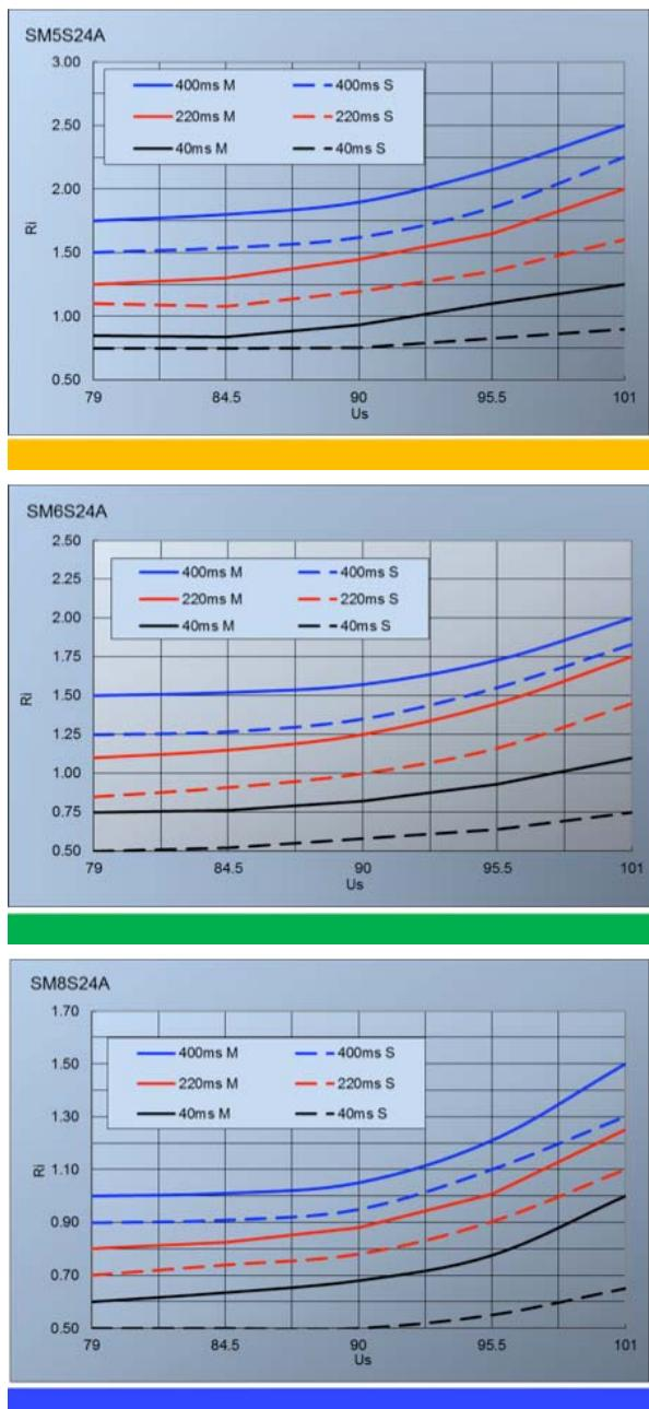
**Figure 5** Capabilities of Vishay's SN5S24A under the new load dump test conditions. Suffix "M" lines are multiple pulses using the new test condition standards (ISO-16750-2). Suffix "S" lines are single pulses as defined by the old test condition standards (ISO-7637-2).
