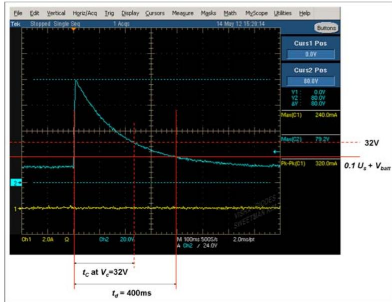
**Figure 1** Input waveform of an ISO-16750-2 pulse: 5A, 79V  $U_s$ , 400ms pulse width condition
