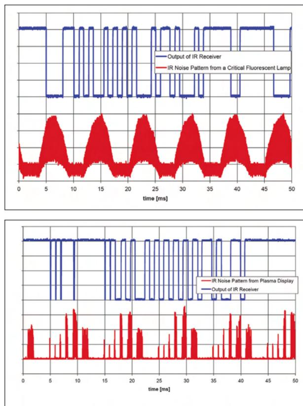
**Top, Figure 4.** The AGC1 receiver output when the same RC5 signal is being received in the presence of a strongly modulated fluorescent light. **Bottom, Figure 5.** The AGC1 receiver output when receiving the same RC5 code plus noise from the plasma television in which it is assembled.
