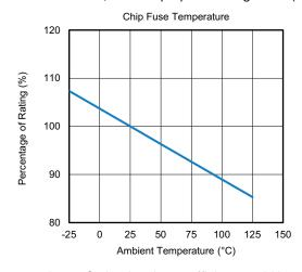
For example, if the ambient temperature is 60  $^{\circ}$ C, the derating coefficient would be 95 %.
