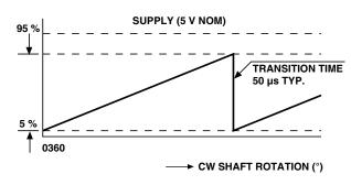
MODEL: 601 HE when pin 4 connected to 5 V or open circuit
