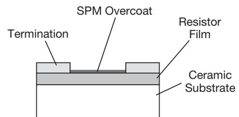
Figure 1. - SPM Construction
