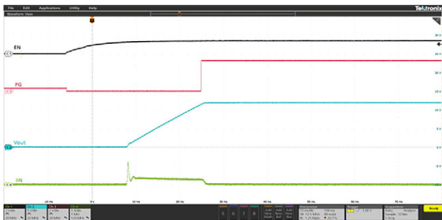
Fig. 50 - Power Start-Up With V IN Ramp
