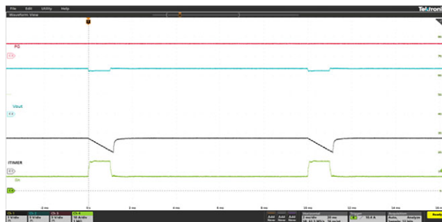
Fig. 30 - Transient Overcurrent Blanking Timer Response V_{IN} = 12 \text{ V} , CITIMER = 3.3 \text{ pF} , C_{OUT} = 220 \mu\text{F} , R_{ILM} = 680 \Omega , I_{OUT} ramped from 7 A \rightarrow 15 A \rightarrow 7 A within 1 ms
