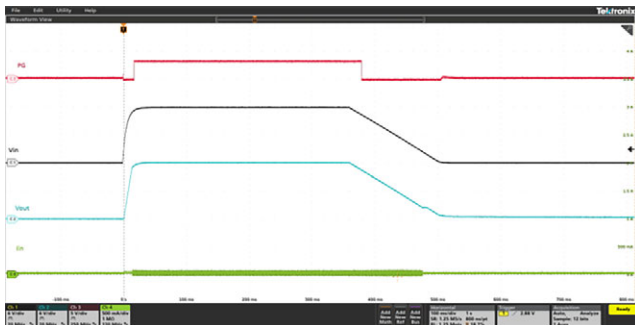
Fig. 20 - Power Up and Down With Input Supply V_{IN} = 22\text{ V} , C_{OUT} = 22\text{ }\mu\text{F} , C_{SS} = 3.3\text{ nF} , VEN/UVLO ramped from 0 V \rightarrow 12 V \rightarrow 0 V
