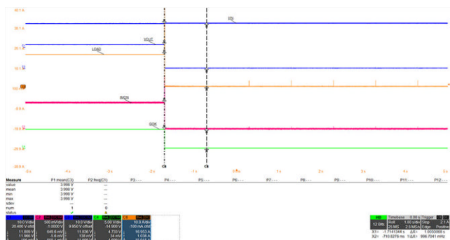
Fig. 25 - SiC32306 Auto Retry after 1 s during short circuit at the outputs
